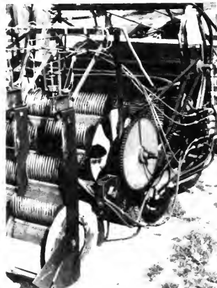
The working gears and teeth of J. S. Norton's dry picking machine.
